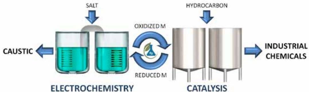
We've pioneered a new technology platform that combines electrochemical and catalytic processes to produce caustic soda and a suite of chlorinated chemicals. This membrane based technology avoids chloride gas with a metal chloride reaction between two integrated processes.
